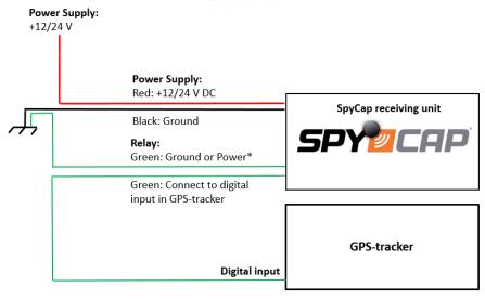
\*Please see the original manual of the GPS-tracker for input settings and setup of alarms.
